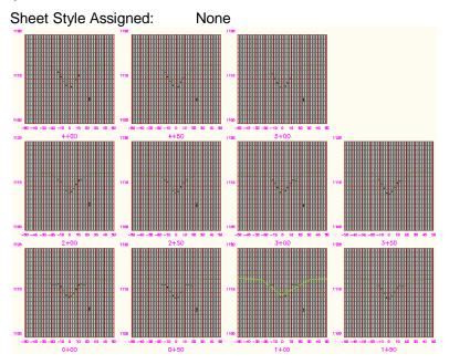
Each group plot style in the North Dakota drawing template has a corresponding sheet style automatically assigned to it, which controls the sheet size and the full sheet grid lines that are plotted. The section view style used in these samples have no grid lines displayed for the individual sections (designated by a No Grid in the style name), since grid lines are provided by the sheet style.
