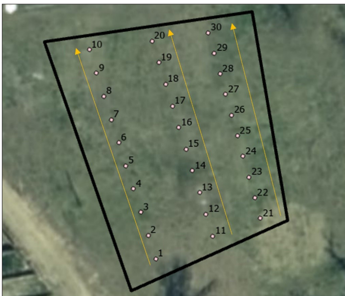
Figure 3. Linear transect is a systematic data collection with a defined spacing between points and transects.
