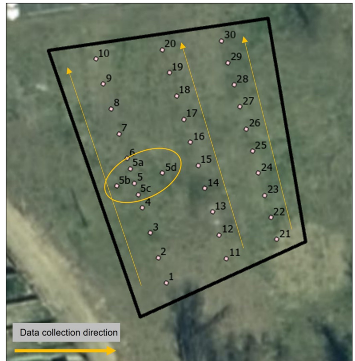
Figure 4. Modified linear transect is a detailed systematic data collection with the ability of capturing anomalies along the transects
