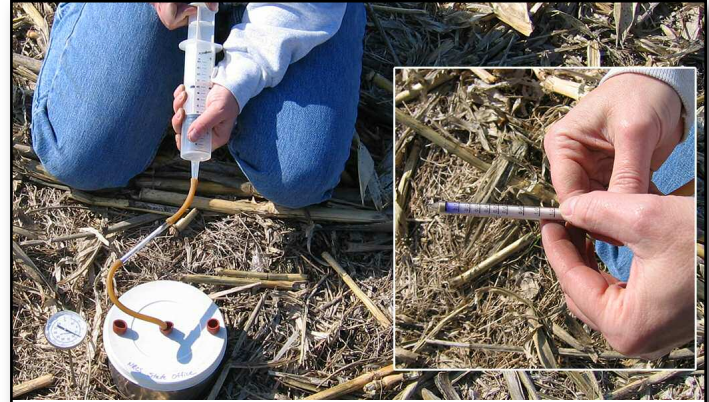
Figure 1. Draeger-Tubes® are used to measure CO 2 released from the soil surface as an indicator of decomposition and soil respiration.
