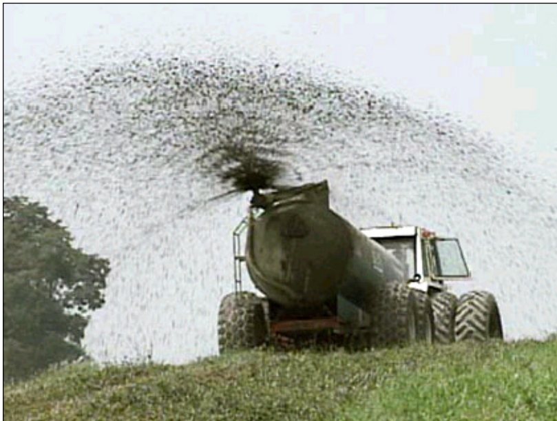
Throwing manure into the air when spreading can increase odors and complaints from neighbors
