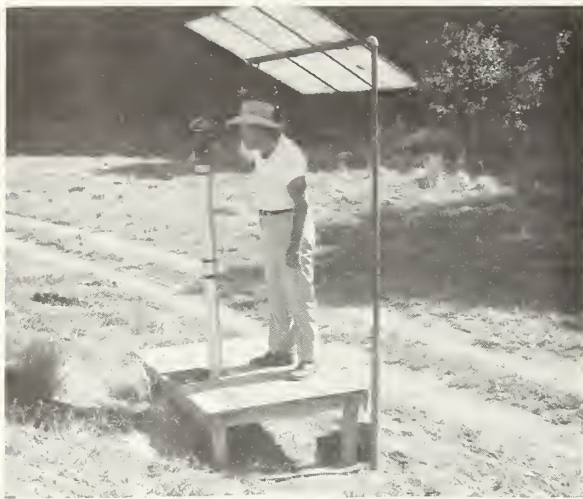
FIGURE 2.—Engineer's level mounted on fixed-pipe unipod. (Upper 2-ft section of pipe can be removed to lower instrument.)
