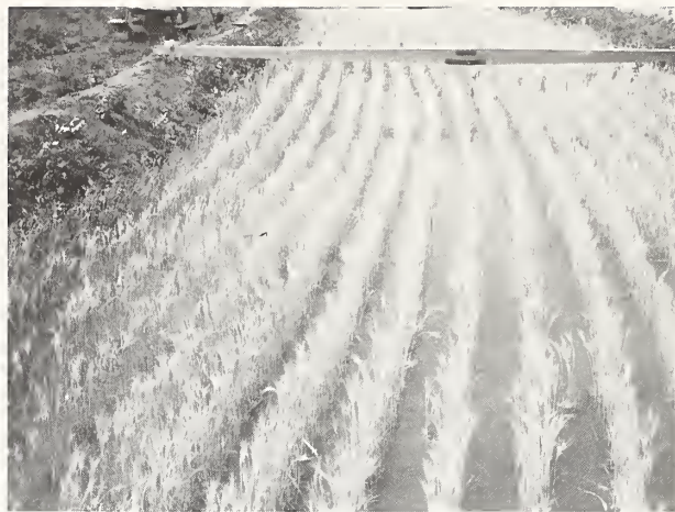
FIGURE 9.—Wheat in reach B of channel FC 29 during flow of 4.1 ft 3 /s with depth of about 8 inches, experiment 3.
