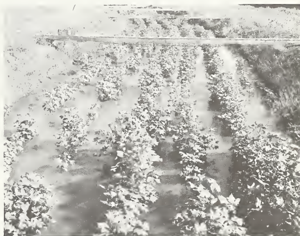
FIGURE 36.—Cotton in reach A of channel FC 29 during flow test 1, experiment 4. (Water depth is about 3 inches.)
