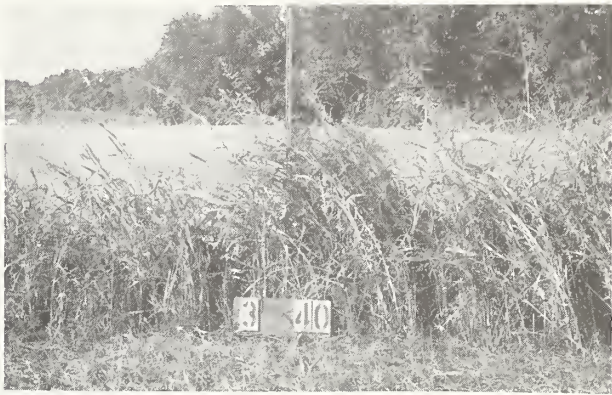
FIGURE 43.—Sudangrass across reach B of channel FC 30 after tests, experiment 6. (Grass in foreground was cut to show 3-ft-wide strip against background.)
