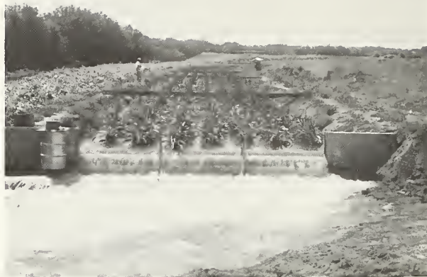
FIGURE 3.—Outlet of channel FC 29 during flow of 31.8 ft 3 /s with the end sill in place, experiment 2. (Top of sill is 0.8 ft above channel grade at outlet.)
