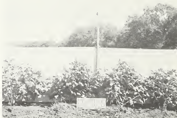
FIGURE 40.—Cotton across center of reach B of channel FC 29 after tests, experiment 6. (Plants in foreground were removed to show height and density of stand.)
