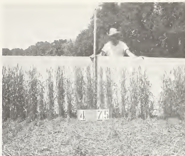
FIGURE 16.—Wheat across center of reach C of channel FC 29, experiment 5. (Plants in foreground were cut to show height and density of stand.)
