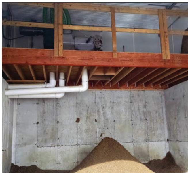
A manure separator removes the manure solids for use as animal bedding or compost.
