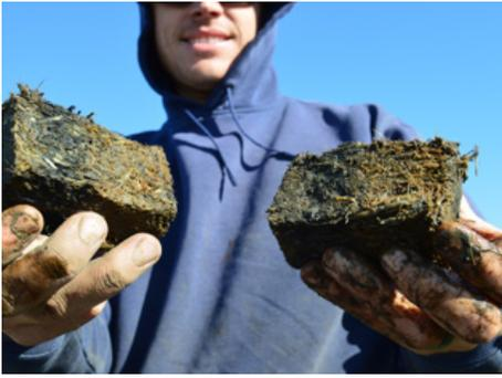
The “brownie” method is one of the best ways to accurately collect bulk density samples. The bulk density data is used to calculate how much carbon is stored in the soil.
