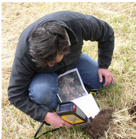
State Soil Scientist Edwin Muniz uses a portable X-ray Fluorescence analyzer in the field.
