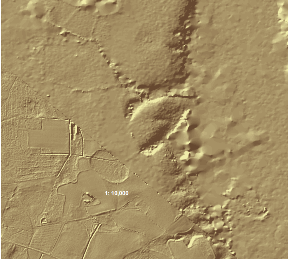
Figure 1. —Hillshade derivative example of a 3m resolution DEM comprised of LiDAR data from two different sources.
