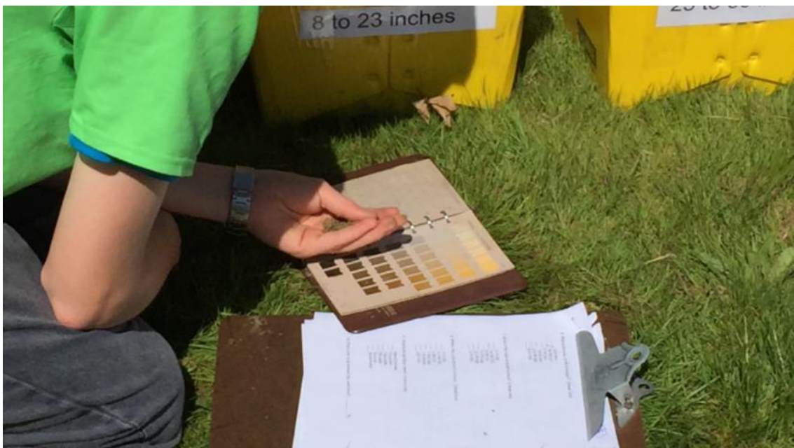
A Munsell color book is used to identify the color of each layer.
