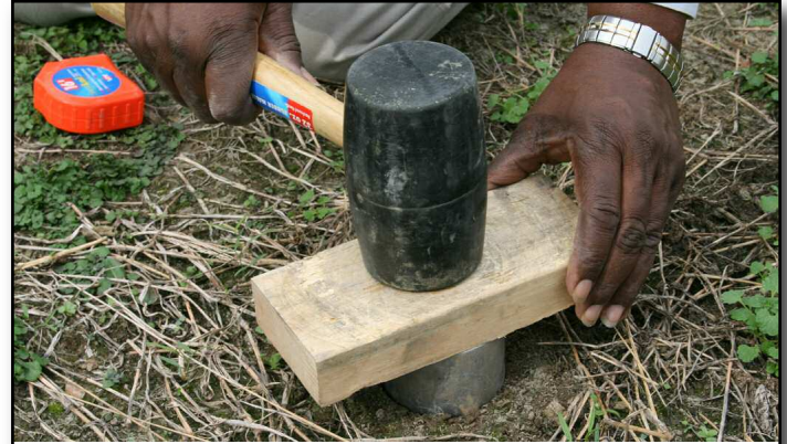
A three inch diameter ring is hammered into the soil to collect bulk density samples.
