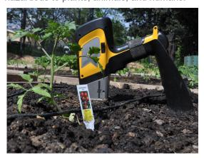
The portable X-ray Fluorescence (PXRF) analysis can determine the concentration of lead and other trace metals onsite; the spatial variability and presence of any "hot spots," and whether there is a need for different use and/or management.
