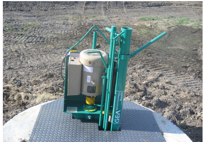
Figure 3. Liquid manure pump for moving water out of the SSB to a holding pond or vegetative treatment area (See VTA Fact Sheet).
