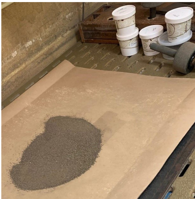
Figure 1B1b2b–5.—Homogenized <2-mm processed soil sample ready for subsampling.
