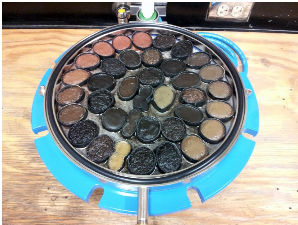
Figure 3C2a-2.—Sieved (<2-mm) soil placed in pressure-membrane extractor.
