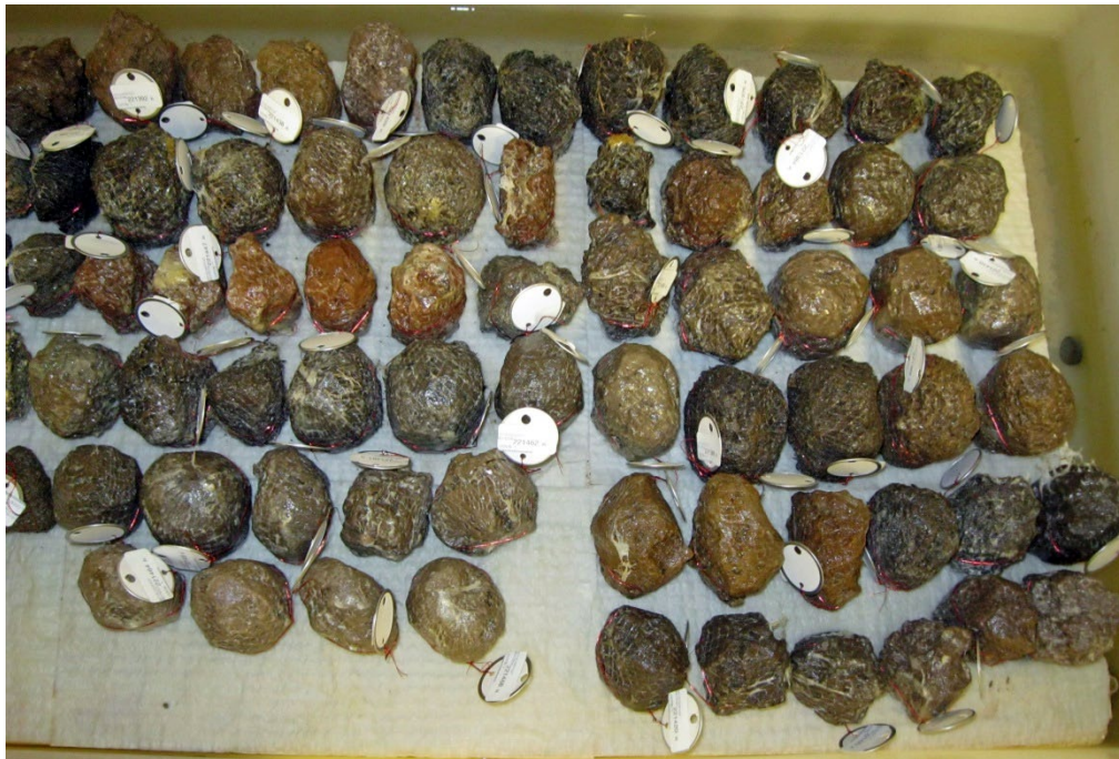
Figure 3C1-1.— After a flat surface on the clod is cut with a diamond-edged saw blade, the clod is placed on a tension table, maintained at 5-cm tension.
