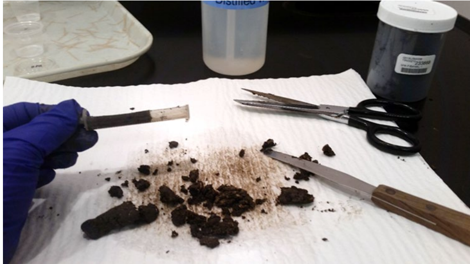
Figure 5C-3.—Sample preparation. Sample segments are packed in syringe.
