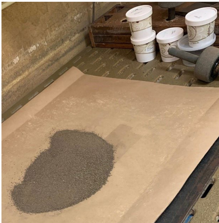
Figure 1B1b2e1–3.—Homogenized <2-mm processed soil sample ready for subsampling.
