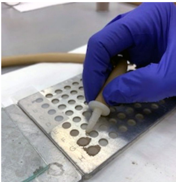
Figure 7A7-6.—Vacuuming excess sample from around wells.
