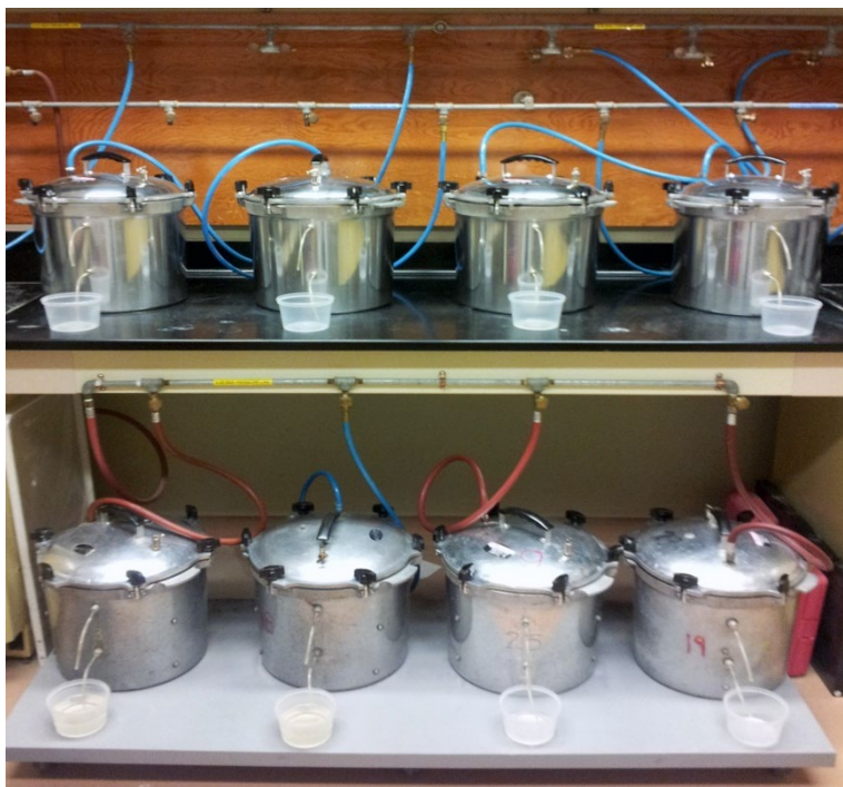
Figure 3C1-3.—Pressure-plate extraction at 33 kPa for clods.
