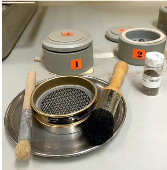
Figure 1B1b2e-2.—Bowls, balls, and sample vial used with planetary ball mill.
