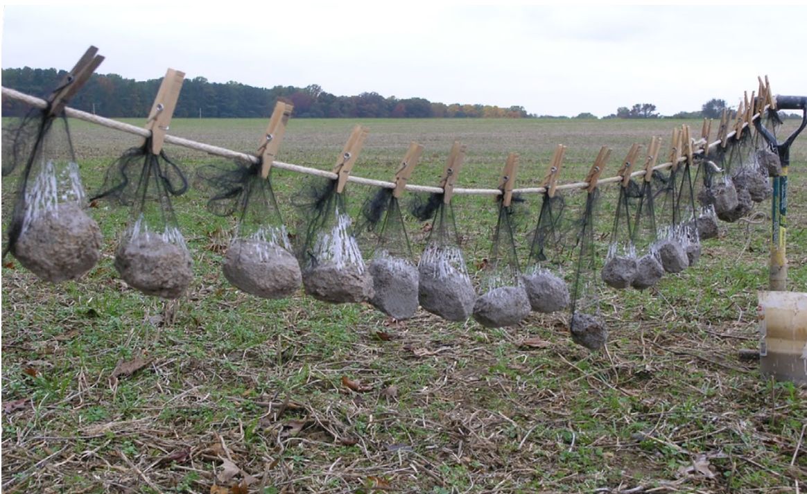
Figure 3B1a-2.—After dipping, clods are tied to clothesline to dry.
