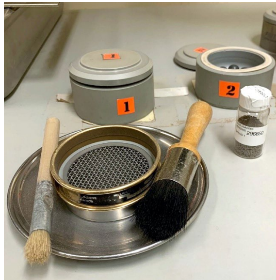
Figure 1B1b2d-2.—Bowls, balls, and sample vial used with planetary ball mill.
