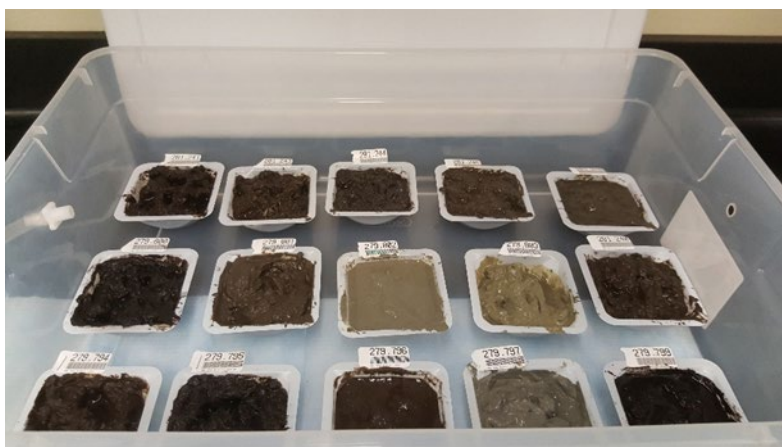
Figure 4C1a1a3–1.—Samples in a humidifier used for measuring oxidized pH.
