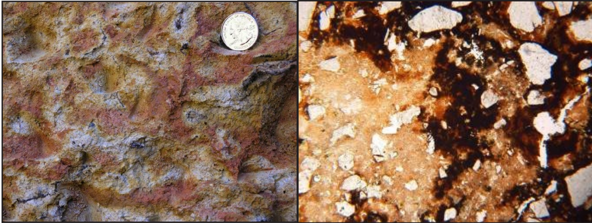
Figure 3E1b–18. —The mottled fabric on the pit face (left) and the thin section of soil fabric from the same horizon (right). These photos illustrate the movement of iron oxides in the soil as it undergoes seasonal saturation and reduction followed by reoxidation. Material is from a Btvx2 horizon of a Fuquay soil.
