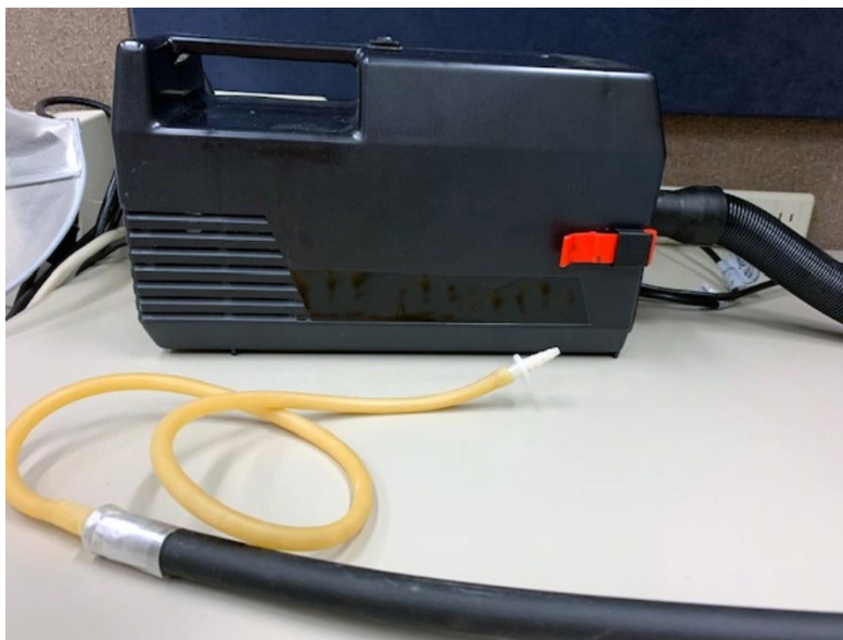
Figure 7A7-3.—Vacuum cleaner with small-end adaptor for removing excess sample from around filled wells on the microplate.
