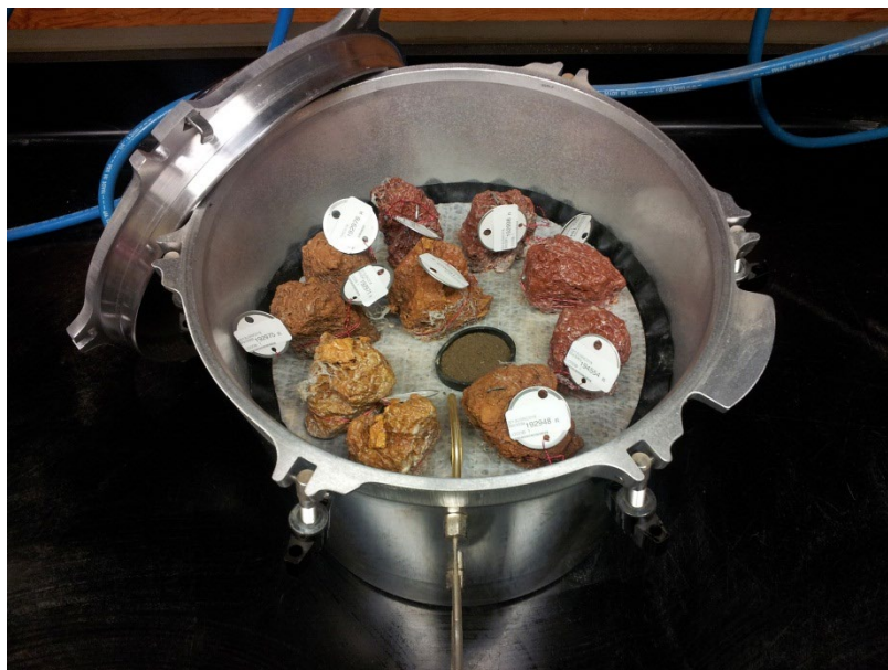
Figure 3C1-2.—Clods in pressure-plate extractor following saturation.
