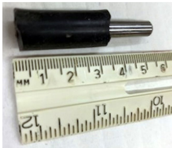
Figure 7A7-2.—Steel press rod used for preparing microplate.
