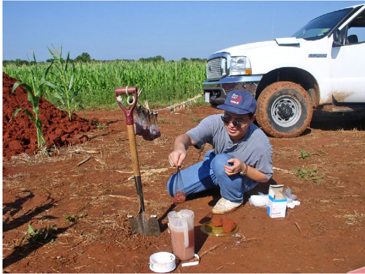
Figure 3B1b-1.—Dipping clods with hairnet in plastic lacquer.
