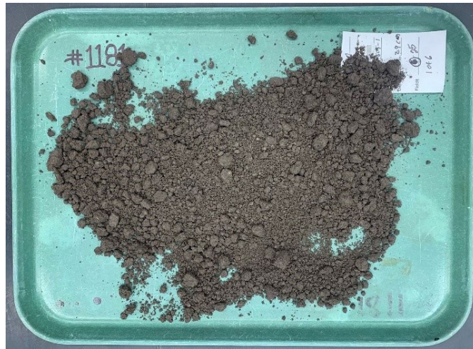
Figure 1B1b2c-3.—Sample prepared for drying with tared tray and sample tag.
