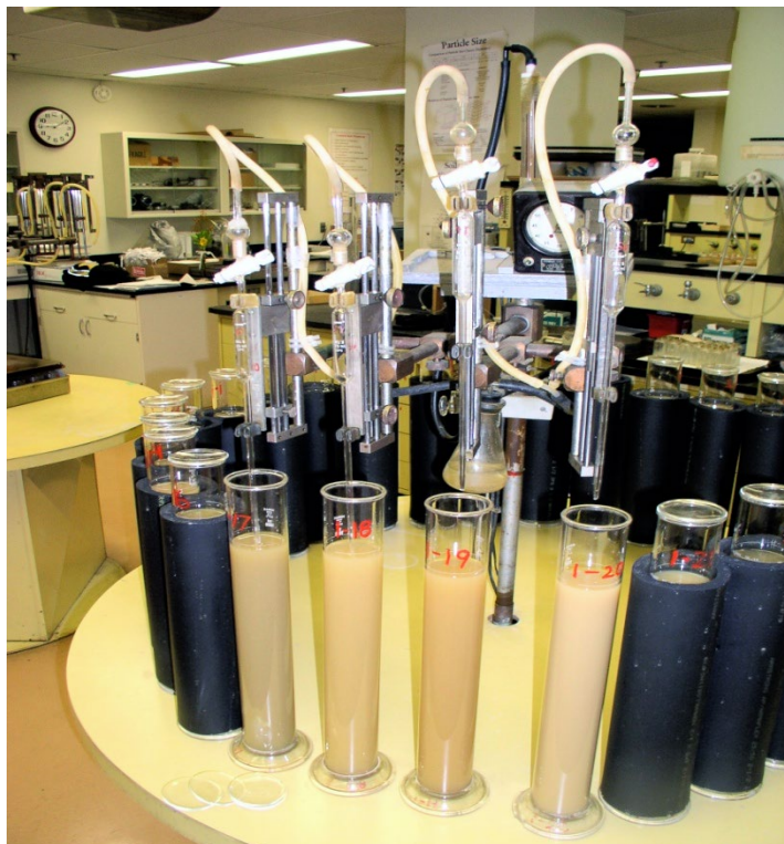
Figure 3A1a1-3.—Shaw Pipette apparatus and Lowy Pipettes used for particle-size analysis at the USDA–NRCS Kellogg Soil Survey Laboratory.
