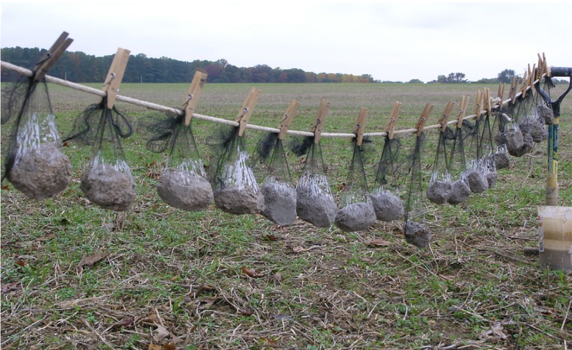
Figure 1A-6.—After dipping, clods are tied to clothesline to dry.
