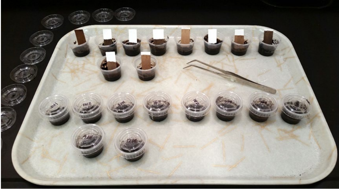
Figure 5B-3.—Day 2 of test, chromatographic paper strips wicking solution.
