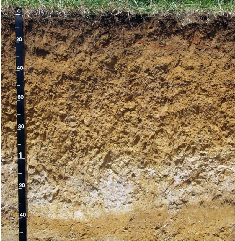
Figure 1A-4.— Photographs are typically taken of a soil profile after the layers have been identified but before the vertical section by the sampling process. Note scale in metric units.
