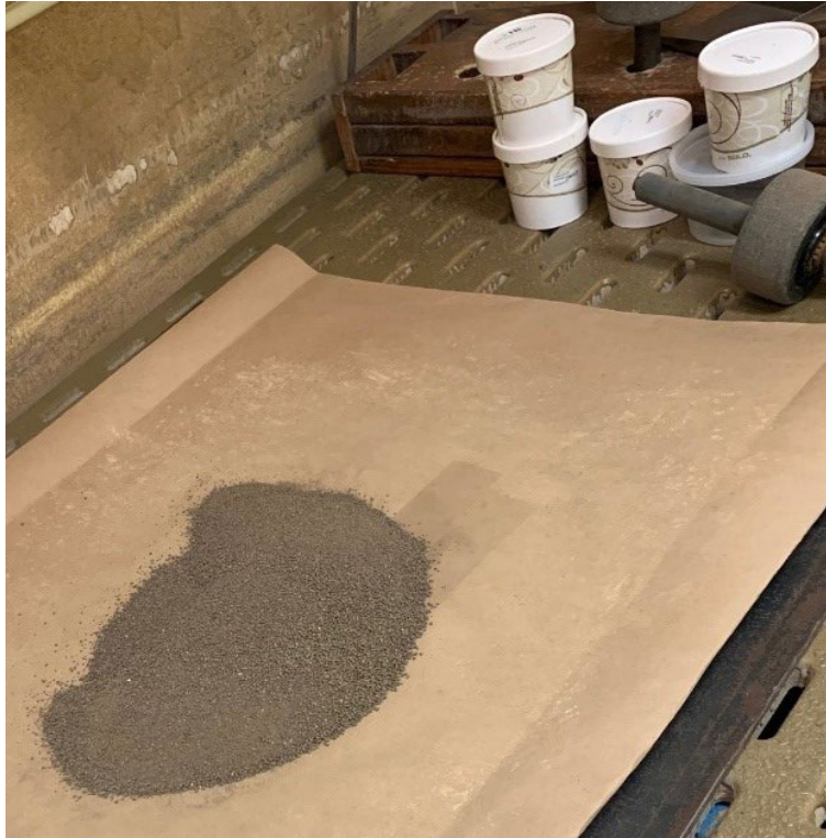
Figure 1B1b2c-4.—Homogenized <2-mm processed soil sample ready for subsampling.
