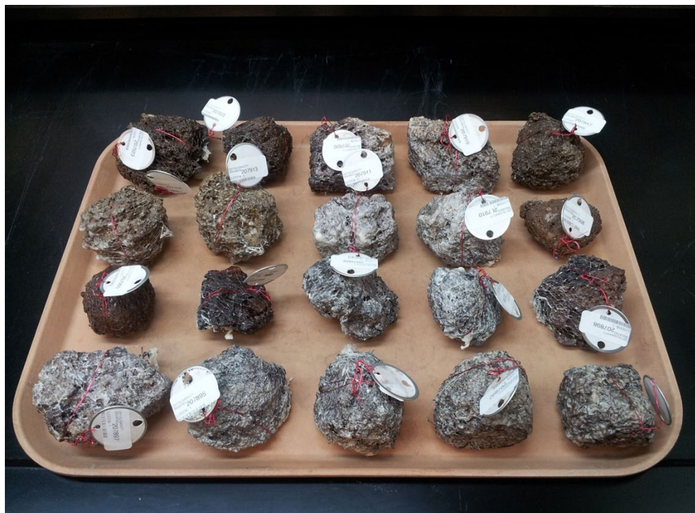
Figure 3B1b–3. —A round stock tag with sample identification number is prepared. The cut copper wire is looped around the clod.
