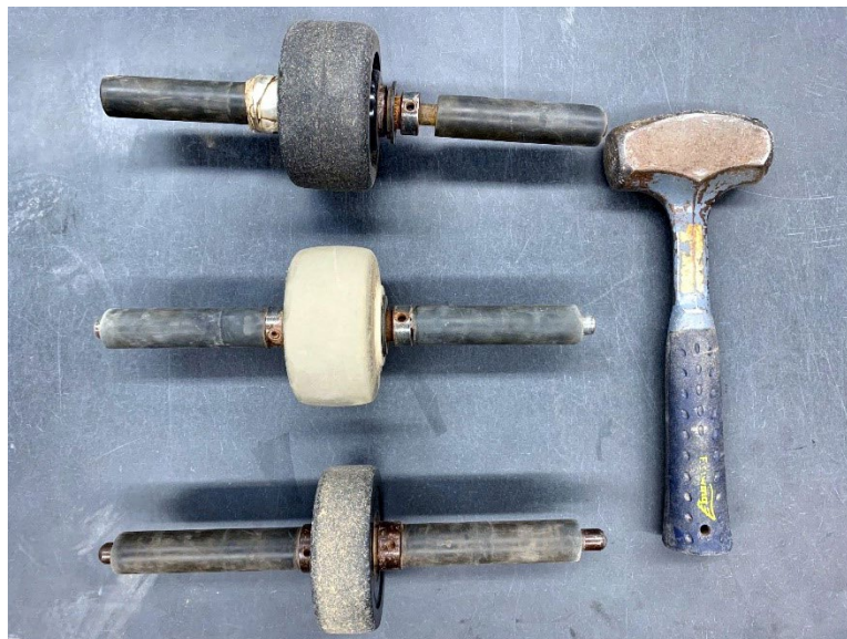
Figure 1B1b2c-2.—Hammer and rubber rollers, custom made for KSSL.
