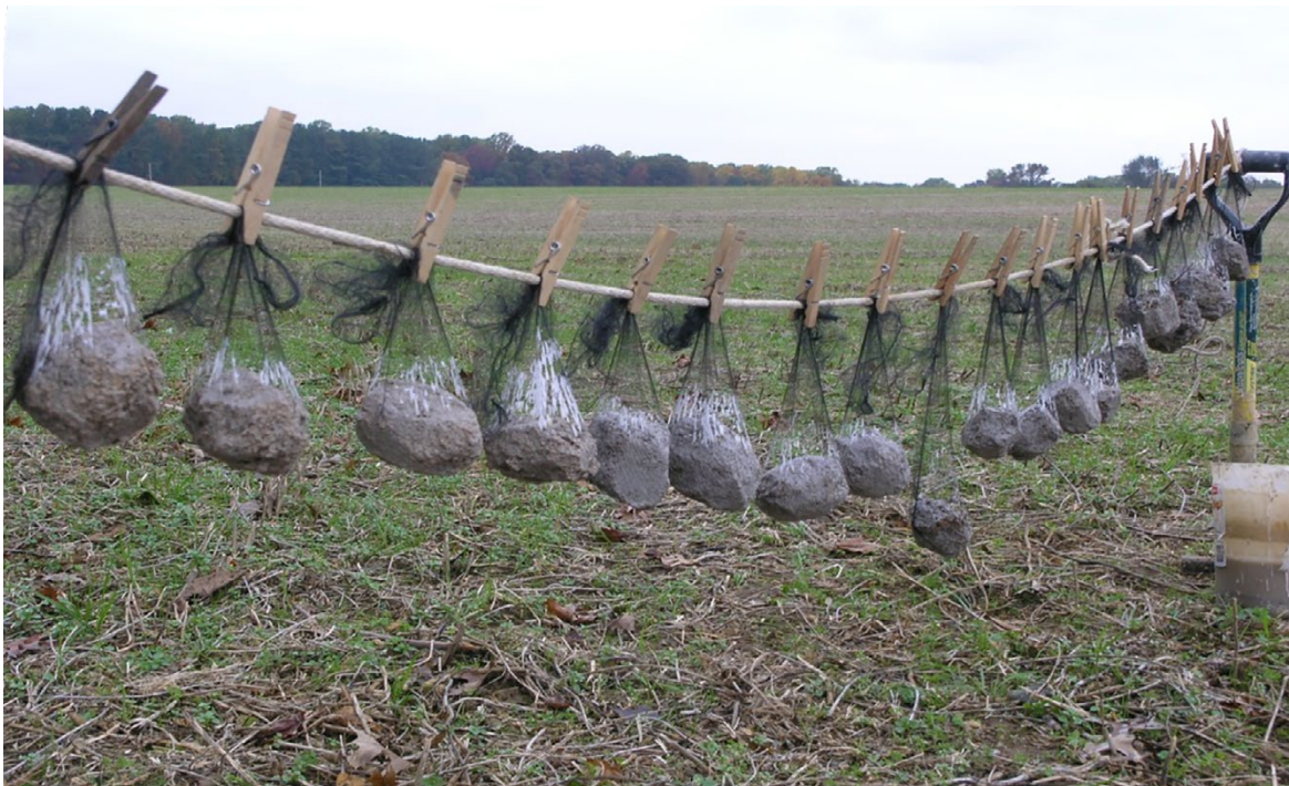
Figure 3B1b-2.—After dipping, clods are tied to clothesline to dry.
