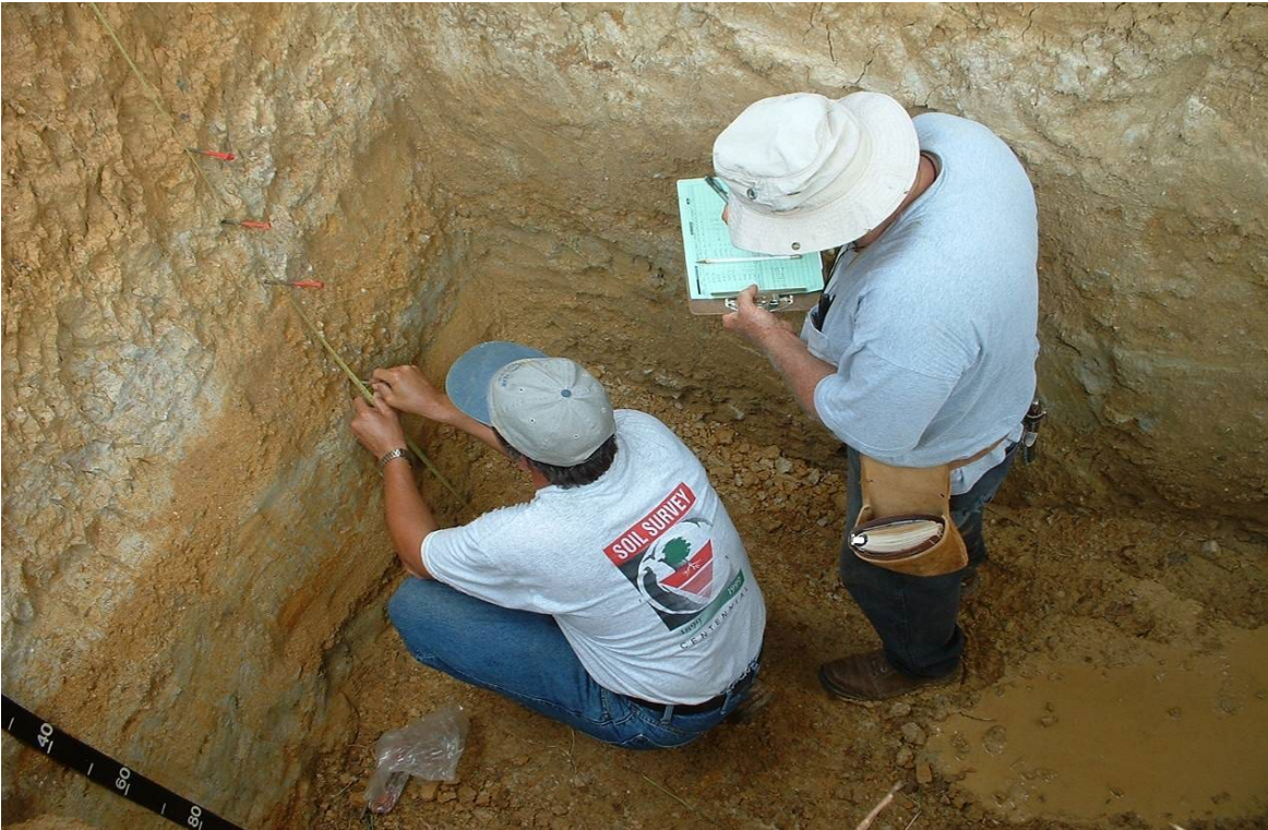
Figure 1A-3.—Soil horizons or zones of uniform morphological characteristics are identified for sampling.
