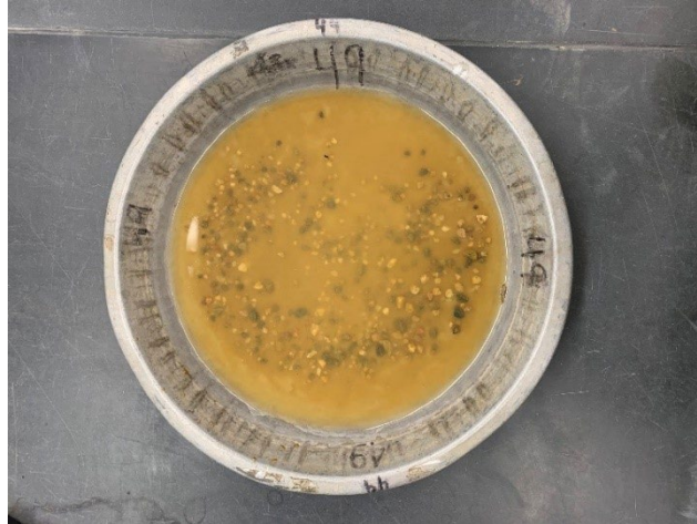
Figure 1B1b2b-7.—Slaking subsample to determine rock fragments from crush-resistant aggregates.
