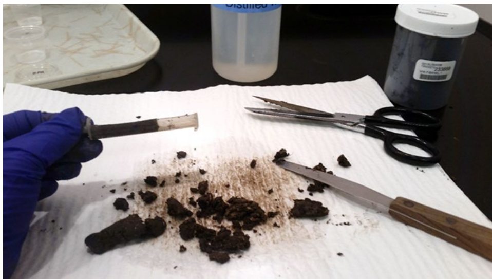
Figure 4C1a1a4-2.—Sample preparation. Sample segments are packed in syringe.
