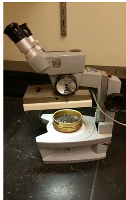
Figure 5C-1.—Stereoscope for examining sample.
