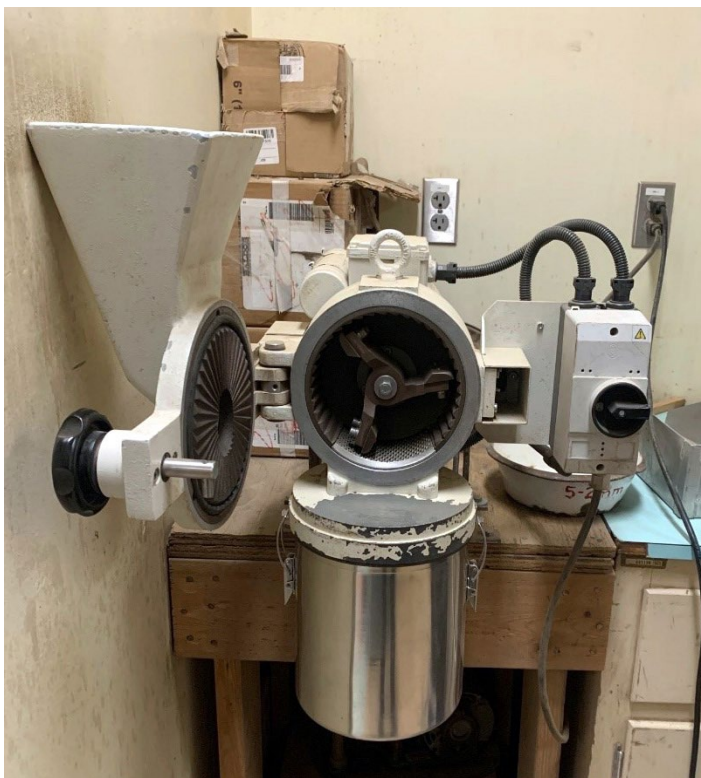
Figure 1B1b2d-3.—Cross beater mill with exchangeable mesh size plates.
