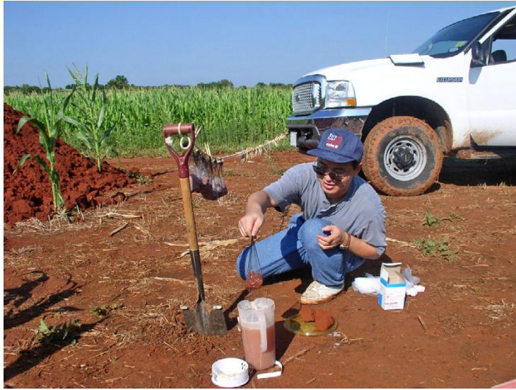
Figure 3B1a-1.—Dipping clods with hairnet in plastic lacquer.
