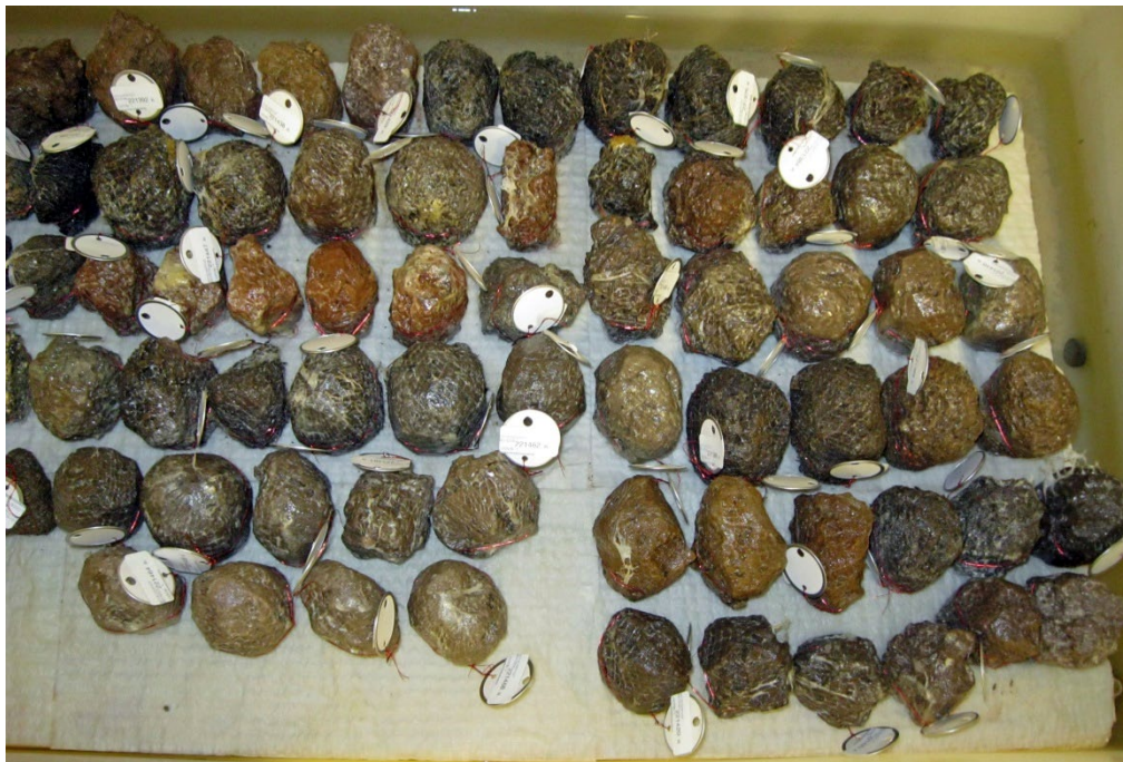
Figure 3B1b–4. —After a flat surface on the clod is cut with a diamond-edged saw blade, the clod is placed on a tension table and maintained at 5-cm tension.
