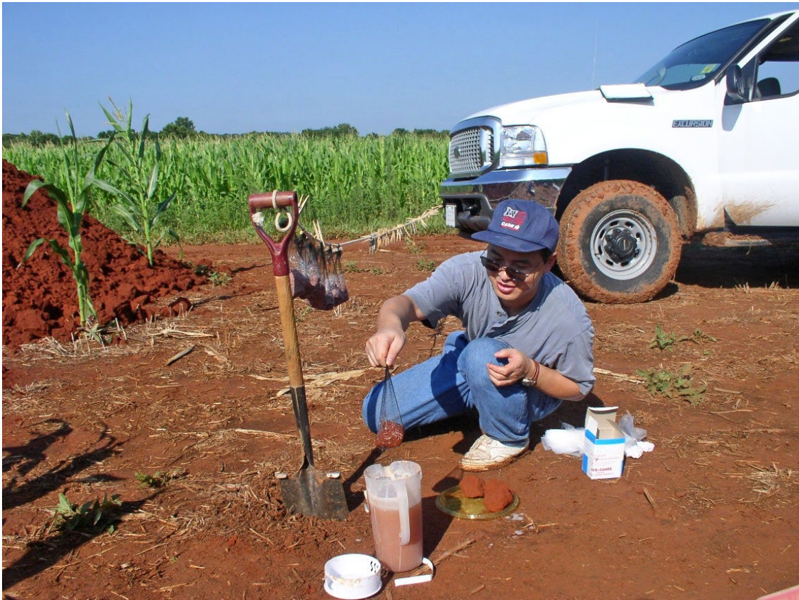
Figure 1A–5.—Dipping clods with hairnet in plastic lacquer.
