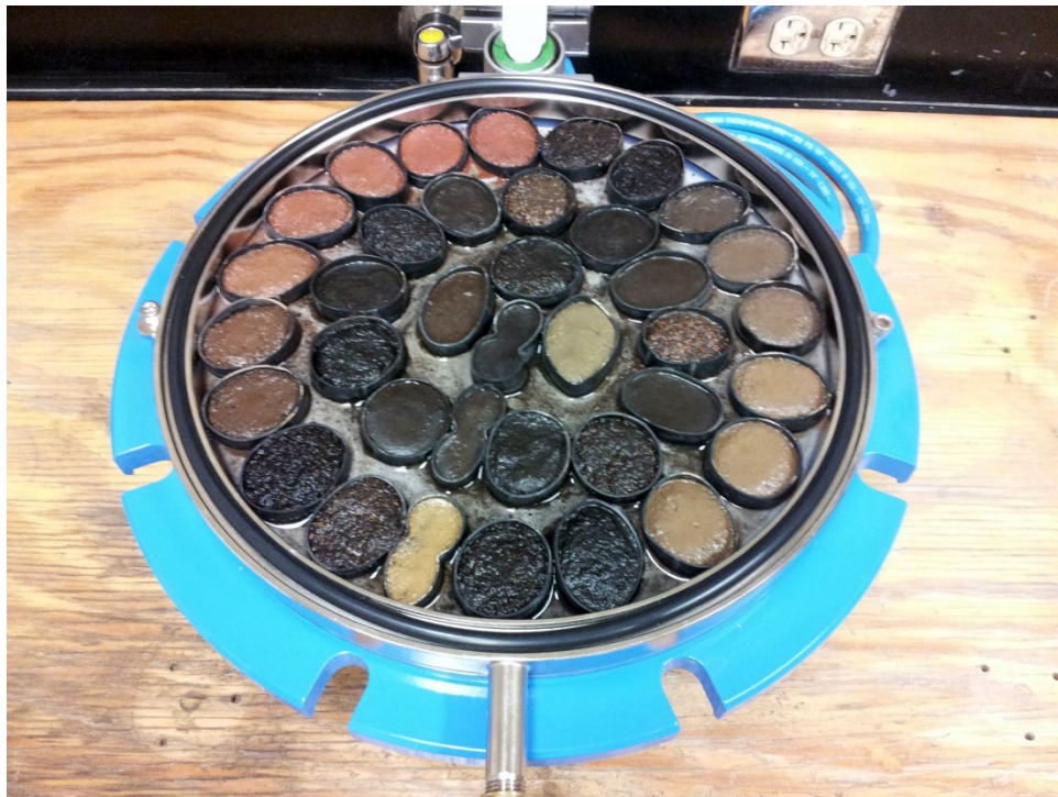
Figure 3C2b-2.—Sieved (<2-mm) soil placed in pressure-membrane extractor.
