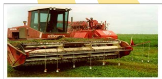
Tractor-pulled and self-propelled haybines mounted with flushing bar devices.
