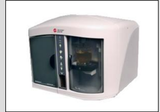
Multisizer IV Coulter Counter used for measuring the concentration and size distribution of collected test aerosols
