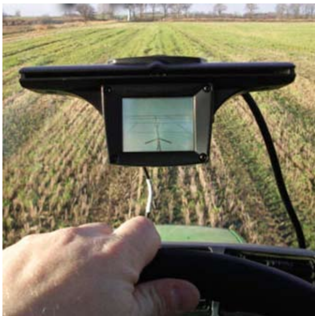
Figure 1 Light bar guidance system
