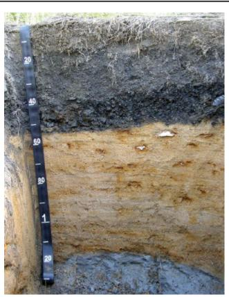
A profile of the Ladyliberty soil series (similar to the one described in the text). Multiple deposits of human-transported materials overlie a naturally deposited gleyed substratum at a depth of 120 cm. The upper 16 cm consists of transported topsoil over transported coal slag with artifacts. Beneath the coal slag, at a depth of 55 cm, is a dredged spoil deposit. (Photo by Richard Shaw)
