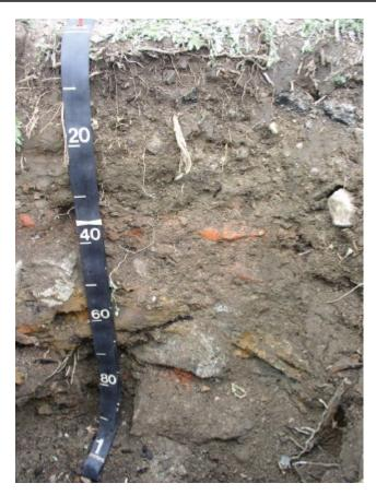
Profile of the Laguardia soil series showing artifacts in multiple deposits of humantransported material. The buried building debris contains brick, concrete, wire, steel, and asphalt. (Photo by Richard Shaw)
