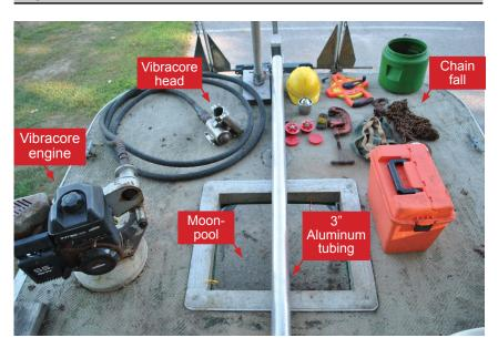
Equipment for vibracore sampling. A vibracore sampler consists of an engine, cable, head, and core barrel. The engines are typically gasoline driven (sold as a device to keep concrete mixed so it does not set). The cable carries the vibrations to the head, which is attached to the core barrel with four bolts.
