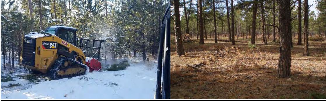
Photos: Masticator at work and after thinning Treatment.
