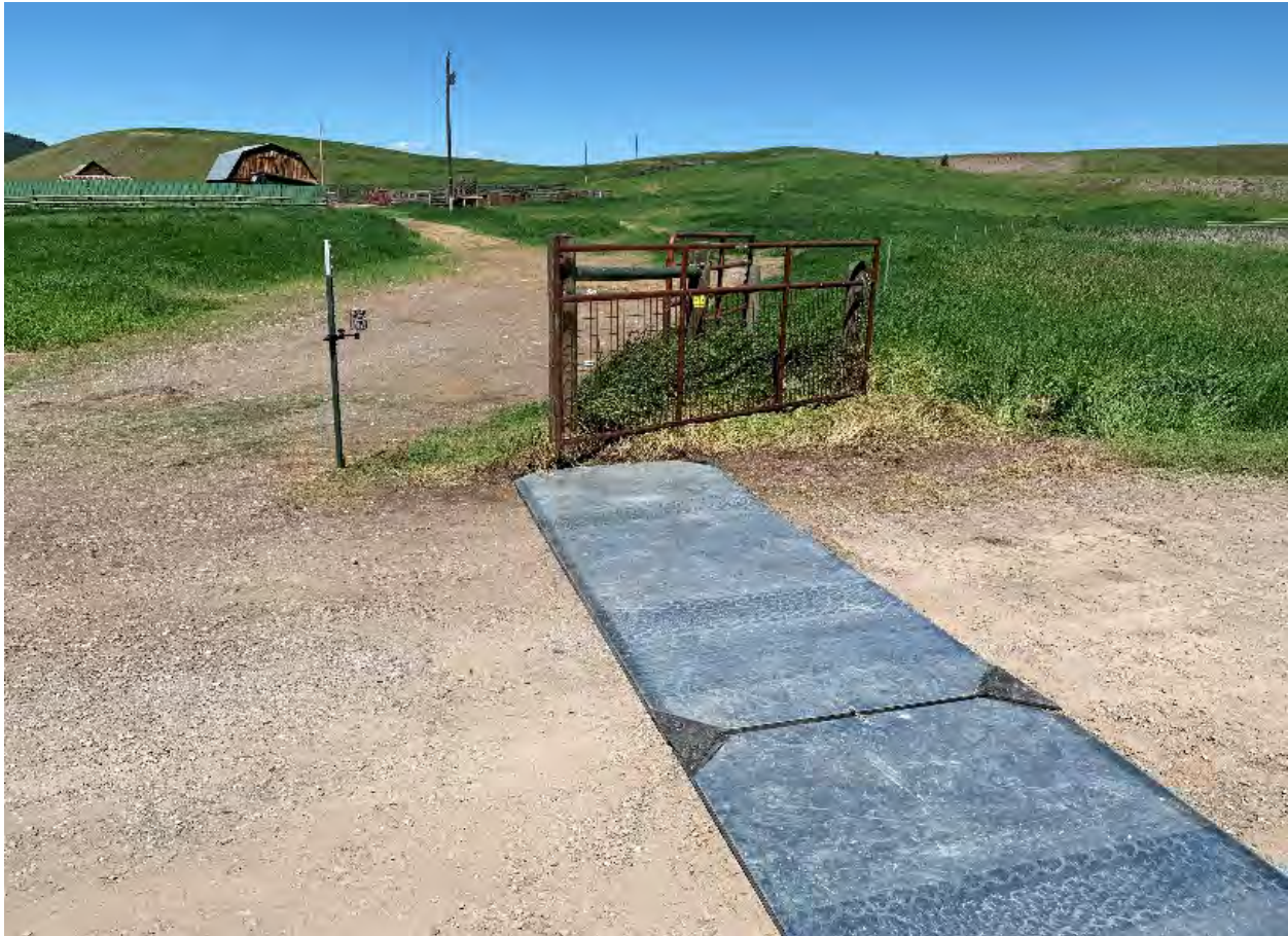
Figure 5. Electrified drive-over mat designed by Brady Stone Fabrication.
