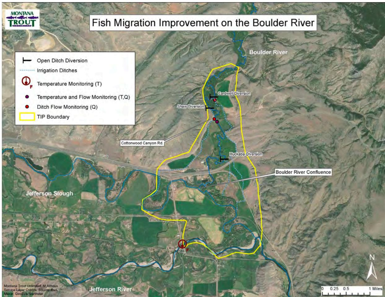
**Figure 2.** The boundary of lower Boulder River irrigated acreage, location of three open ditch diversions, and monitoring sites.
