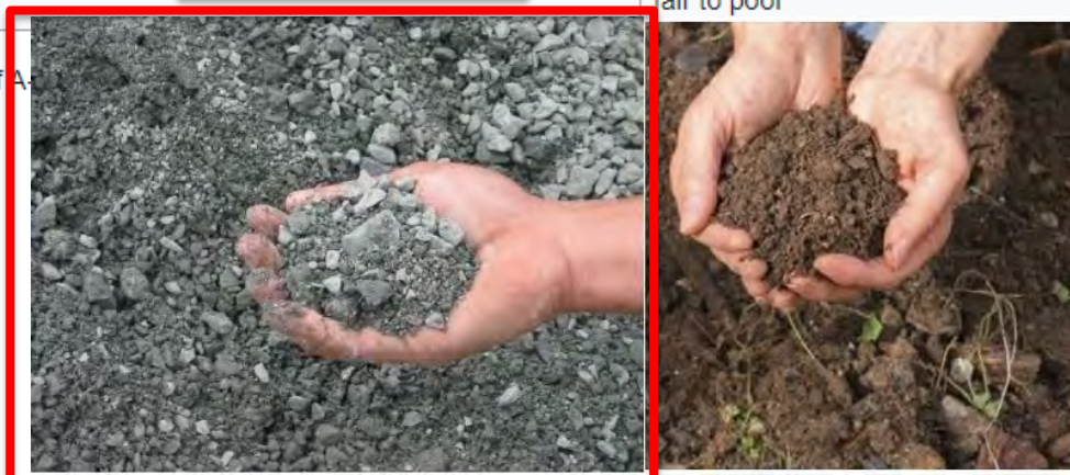
Figures 16 & 17: Pictures of soils. We want the one in the red box. Well graded, multiple size aggregate.
