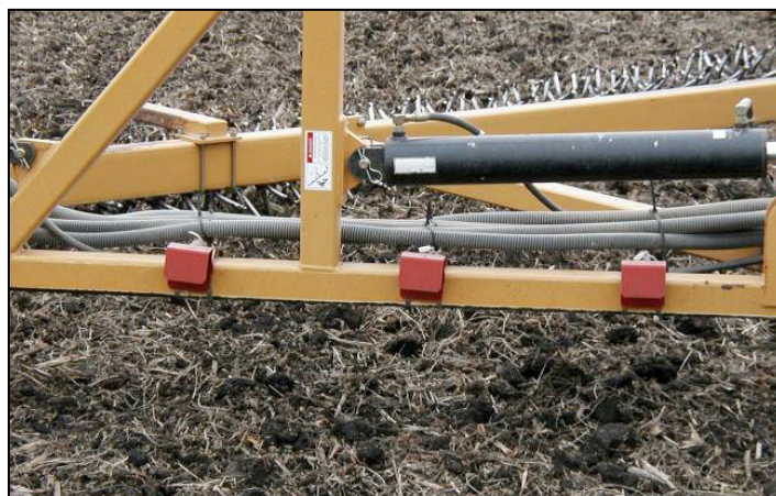
Rotary Harrow Seeding - seed delivery ports
