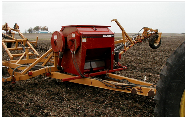
Rotary Harrow Seeding - mounted air delivery seeder in light crop residue
