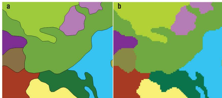
*Figure 1.—(a) An example of the traditional vector-based SSURGO map unit polygon format at 1:6,000 map scale; (b) the corresponding new raster-based Gridded SSURGO (gSSURGO) 10-meter map unit format.*
