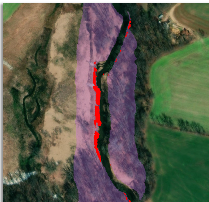
The red areas indicate portions of streambank that have eroded between 2014 and 2019. The shaded area is a legacy sediment terrace.
