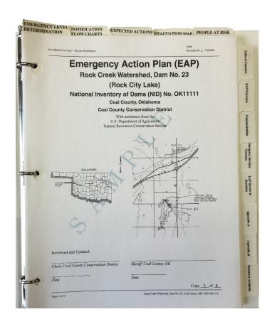
NRCS suggests placing EAPs into three ring binders, with "hot" button tabs across the top and other divider tabs on the side.
