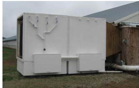
Figure 2.9 Two-stage scrubber using water and an acidic solution developed by USDA/ARS.
