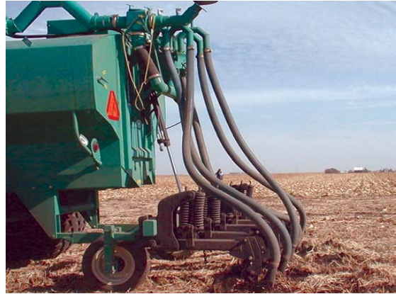
Figure 4.3. Injection of liquid and slurry manure.
