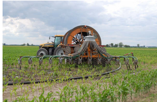
Figure 4.5. Band spreading of manure.
