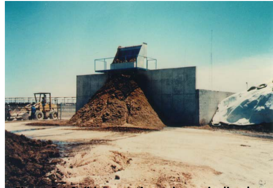
Figure 3.1 Solid separation using an inclined screen separator.
