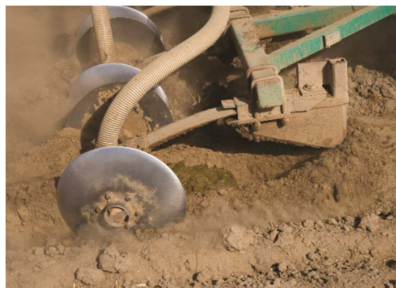
Figure 4.4. Injector unit, which can also be used as a shallow incorporation tool.
