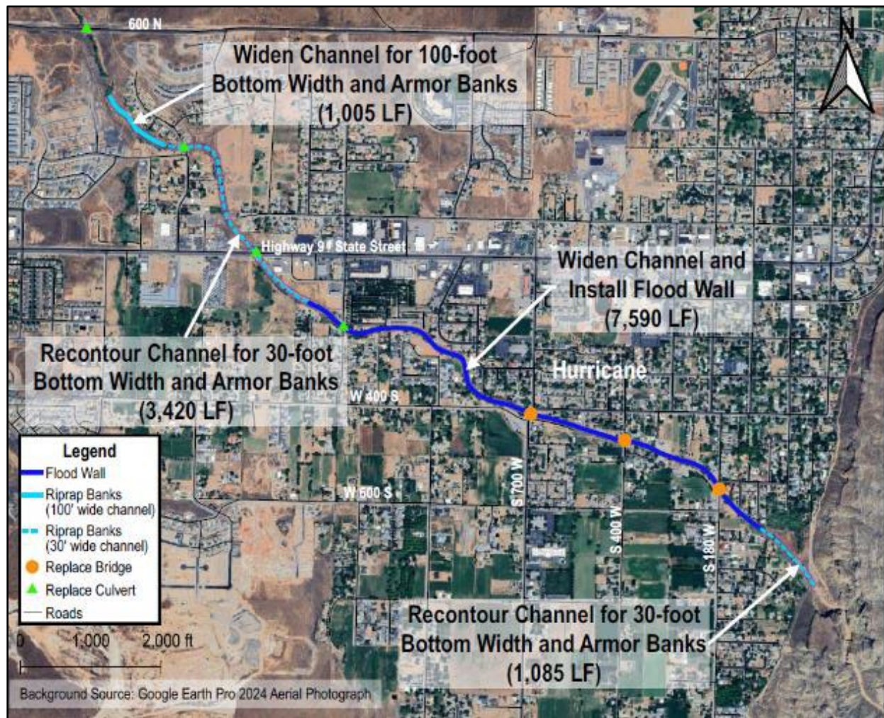
Figure 4-1. Gould Wash Channel Improvements for 8,820 cfs
