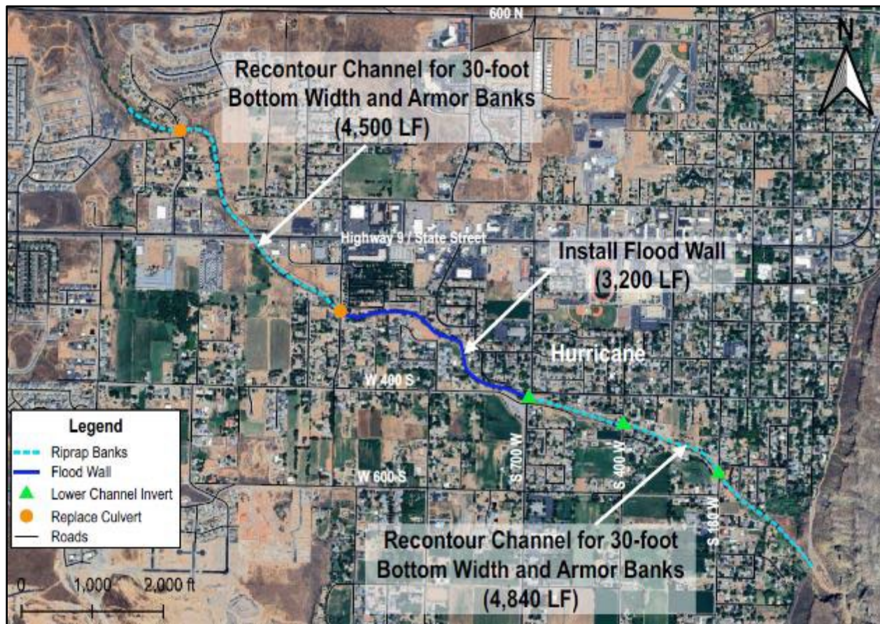
Figure 4-6. Gould Wash Channel Improvements for 3,000 cfs
