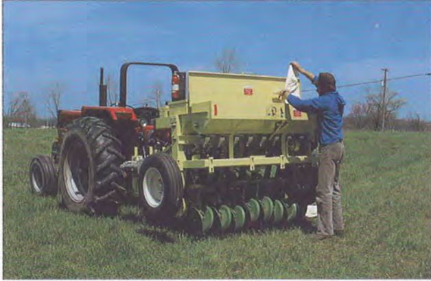
Drills specially designed to plant native grasses can seed into many different types of seedbeds.
