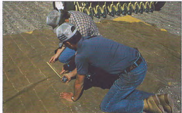
Grass seeding drills can be calibrated by counting the seeds delivered per measured length of row.
