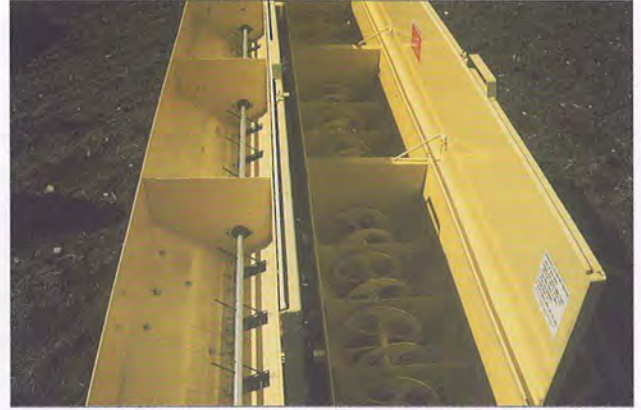
Seed box agitators help to maintain an even flow of native grass seeds to the furrow openers.
