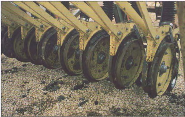
Depth control blades ensure uniform, shallow seed placement.
