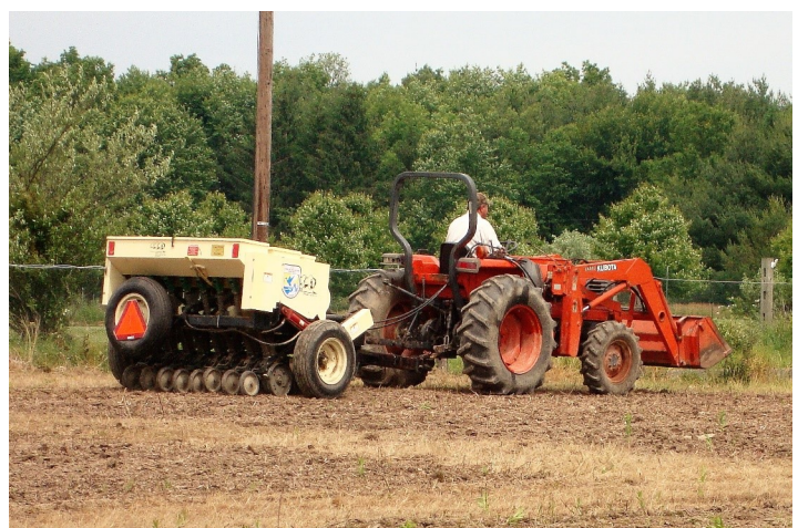
FIGURE 10. Native seed drills are ideal for large planting sites (5+ acres). Typical models have depth controls for optimal seed placement and separate seed boxes for different sizes of seed. Photo: Xerces Society/Kelly Gill
