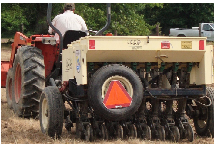
FIGURE 10. Native seed drills are ideal for large planting sites (5+ acres). Typical models have depth controls for optimal seed placement and separate seed boxes for different sizes of seed. Photo: Xerces Society/Kelly Gill
