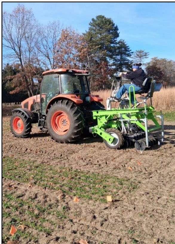
Figure 1. Installation of cereal rye using a Wintersteiger precision plot planter in well-prepared seedbed in fall 2025.
