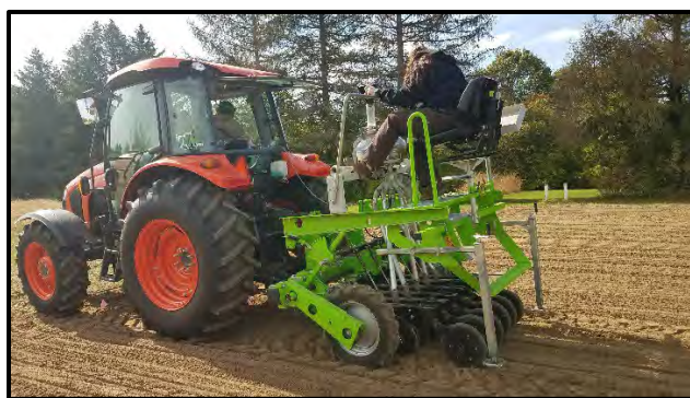
Figure 1. Installation of cereal rye using a Wintersteiger precision plot planter in well-prepared seedbed.
