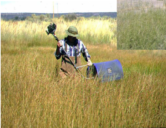
Seed collecting with racquet and hopper (above and right), and motorized seed stripper (below). Photos by Scott Jensen and Chris Hoag.
