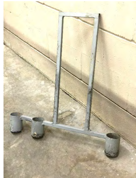
Figure 6. A metal jig welded with sections of 3 to 6-inch pipe can be used to burn holes into weed barrier fabric with a hand torch. Derek Tilley, NRCS Idaho.
