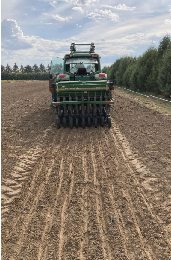
PMC staff seeding National Cover Crop Seed Yield Trial plots. The monocultures were seeded with a Great Plains drill on 7" rows. August 2025.
