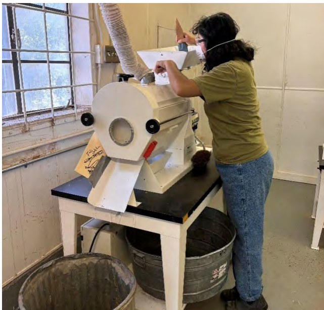
PMC intern, Jenny Salguero processing western stickseed through a laboratory brush machine.
