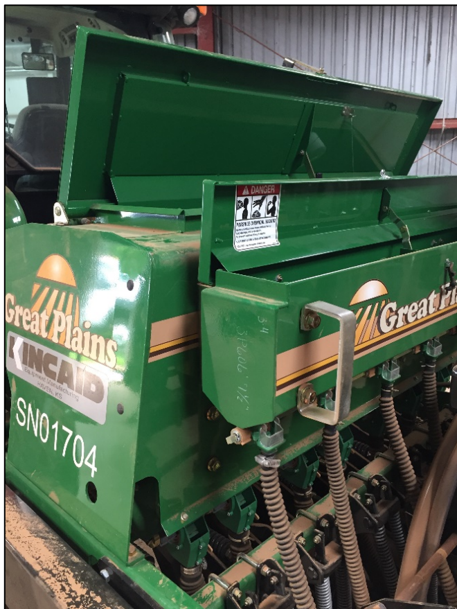
Figure 1. Grain drill with optional small seed attachment included on the back of the large seed hopper
