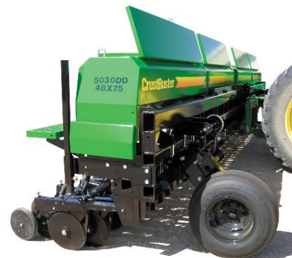
A grain drill with a standard seed box, note the V openers and press wheels with no fluted coulter.
