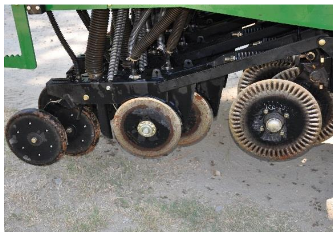
The front fluted coulters of a no-till drill slices an opening through hard sods for the “V” openers, seen middle, to open and deposit seed. The spring loaded press wheels then seal the opening.
