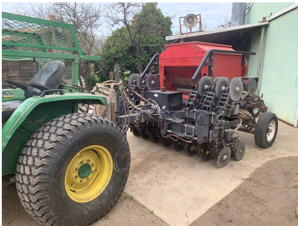
Fig. 1. Custom cover crop seed drill designed and built by Leslie Miller, cover crop and orchard cover crop farmer. 2020.
