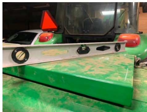
Fig. 10 – Level planter on the ground
