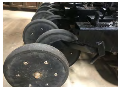
Fig. 8 – Closing or packing wheels can be adjusted for good seed to soil contact.
