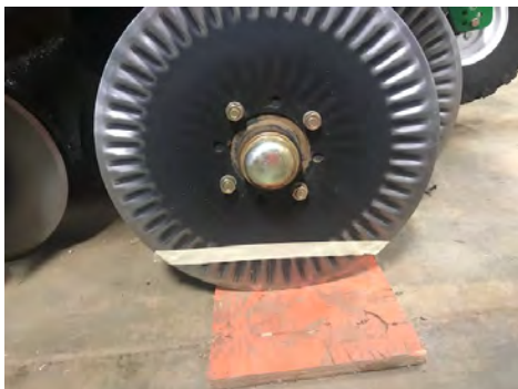
Fig. 7 - Setting correct seed depth on coulters Before operation of planter with tape.
