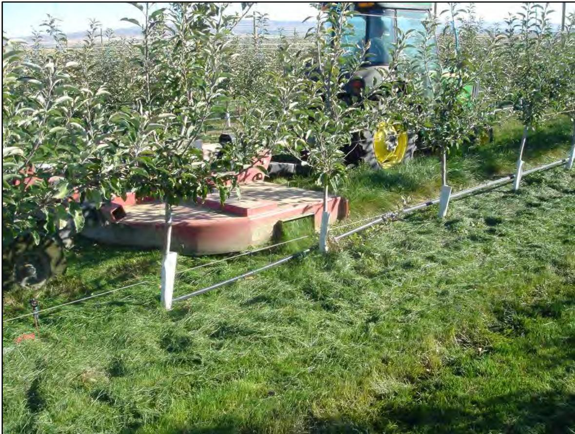
Rotary mower with side delivery distributing drive row vegetation into the tree row. Known as the “mow and blow” management method. D.M. Granatstein.
