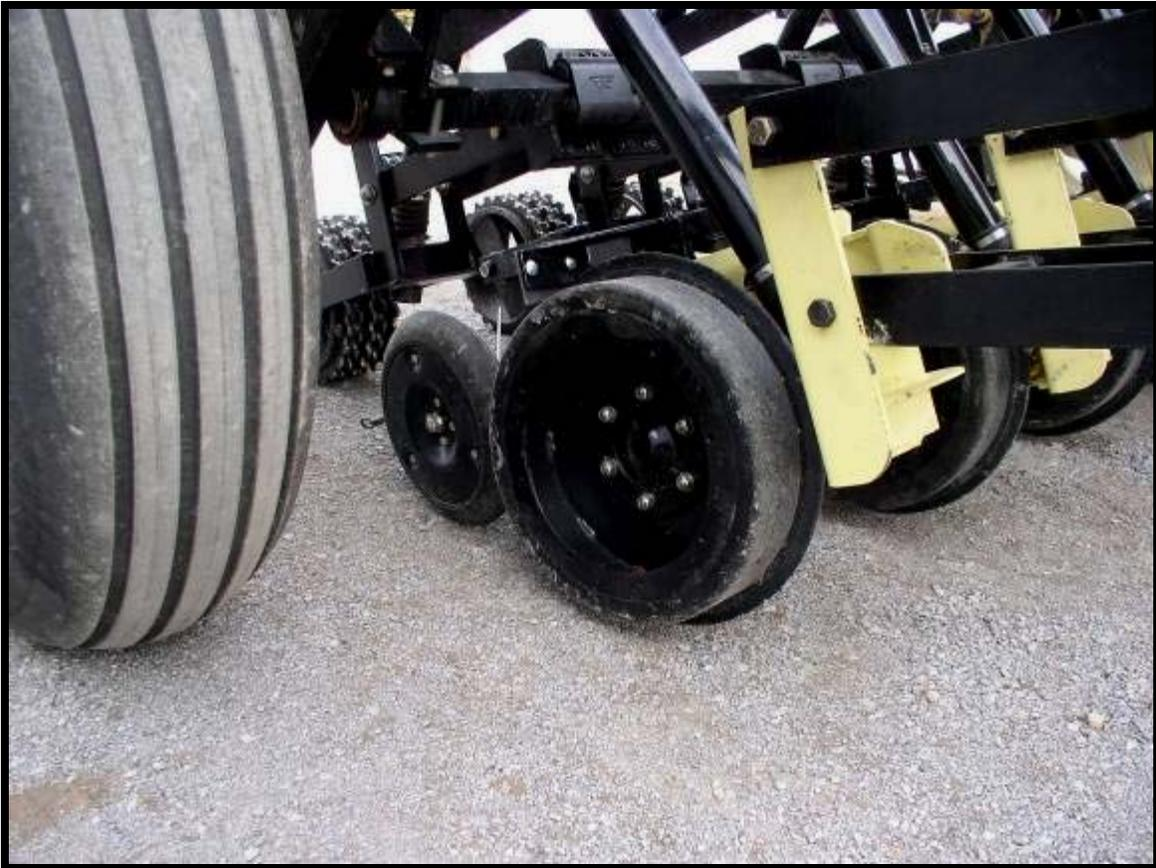
Figure 1. Close-up view of drill seeding unit.
