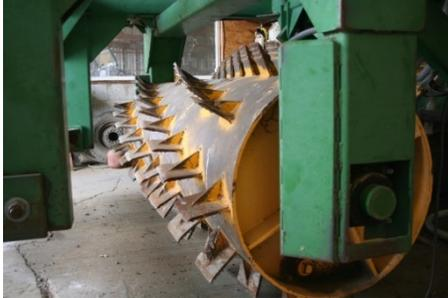
Figure 2. Imprinters (above) and aerators (left) create depressions and microsites that can aid in trapping moisture for seedling emergence. Photos by Kimseed, Australia and Derek Tilley, NRCS respectively.
