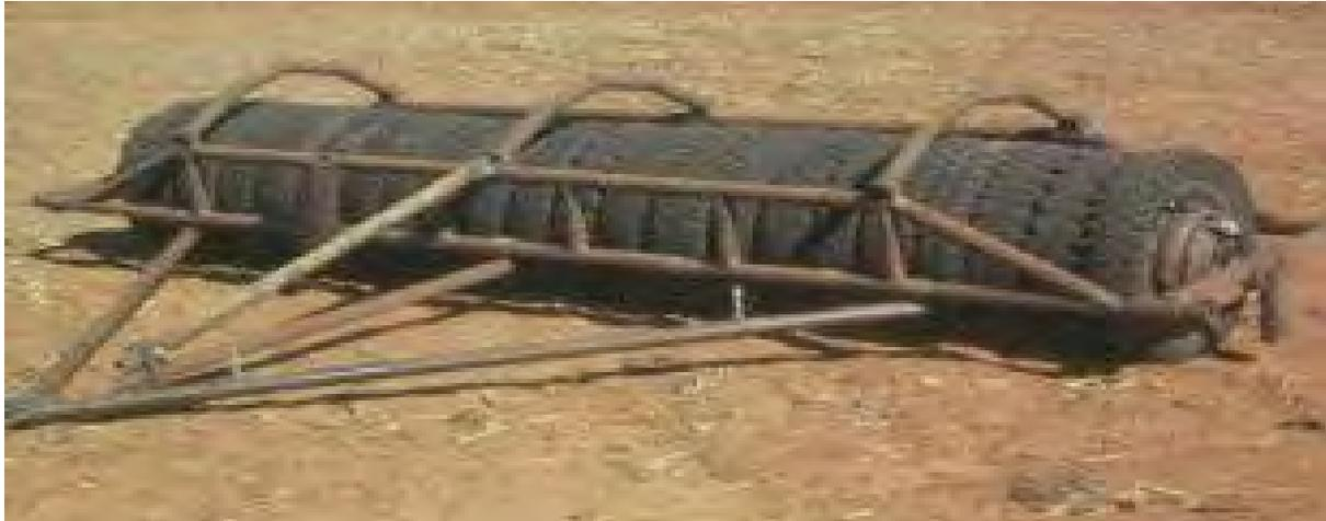
**Figure 9. Shop made rubber tire packer**
