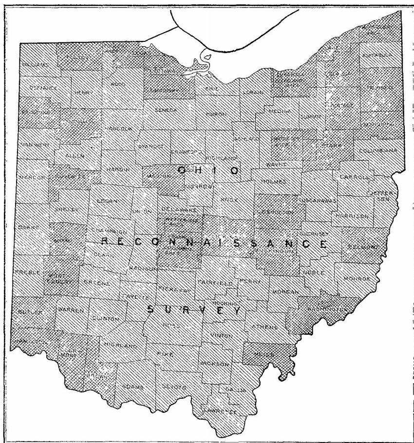
Areas surveyed in Ohio shown by shading. Detailed surveys shown by northeast-southwest hatching; reconnaissance surveys shown by northwest-southeast hatching; cross hatching indicates areas covered in both ways.
