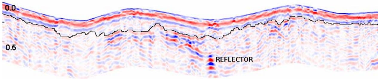
Figure 3. Representative radar profile of an area of Sunapee soil with ortstein. Radar profile obtained with a 400 MHz antenna.
