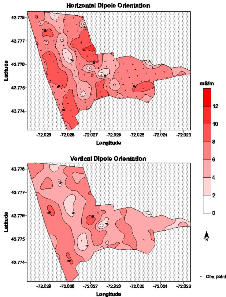
Figure 4. EMI survey of the Mascoma site. Survey was conducted with the GEM300 sensor at an operating frequency of 9810 Hz. All values are expressed in mS/m.
