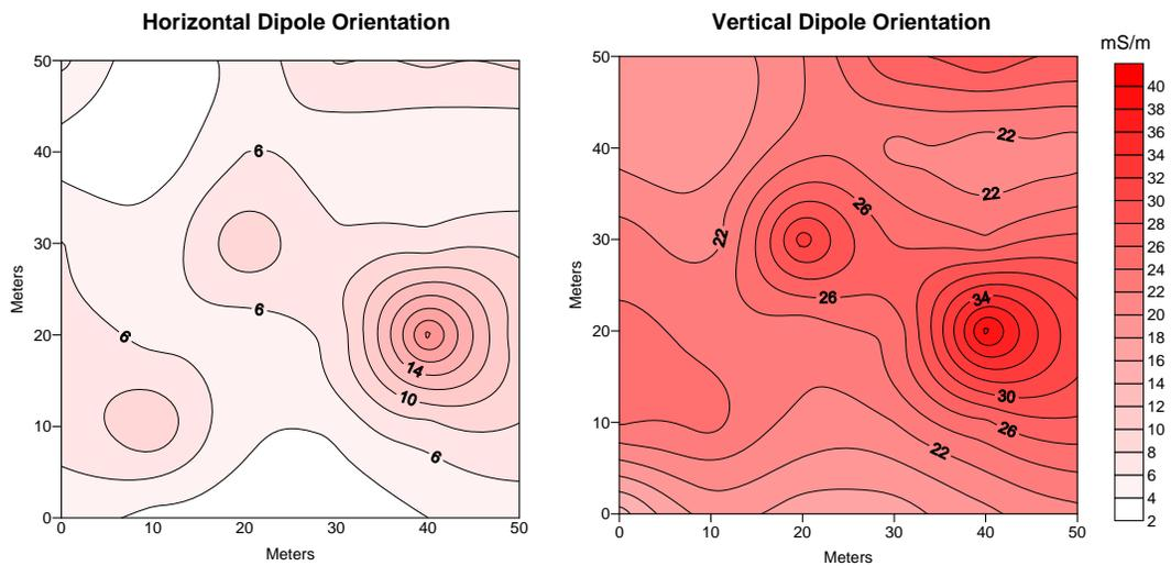
Figure 2 – Spatial pattern of apparent conductivity in an area of Battlerock loam, saline-sodic phase, 0 to 3 percent slopes, measured with the GEM300 sensor at a frequency of 14790 Hz.
