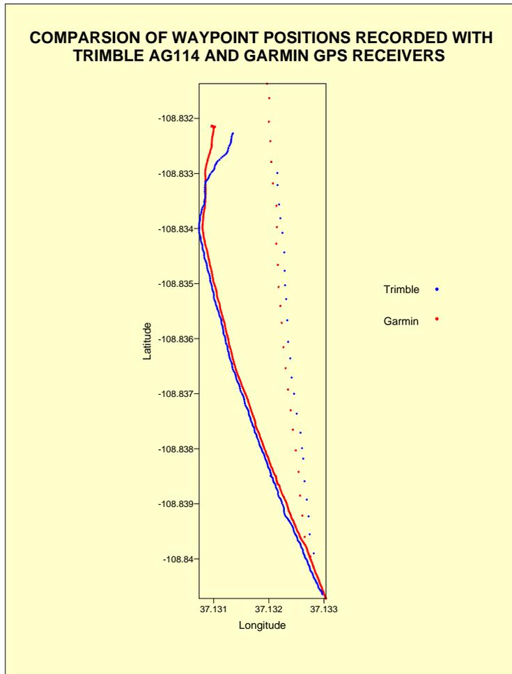
*Figure 5 – Comparison of relative positioning of waypoints obtained with a Garmin GPS Map 76 and Trimble AG114 GPS receivers in an area of Gypsey loam, 3 to 6 percent.*
