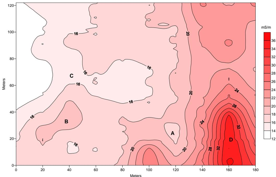
Figure 1 – Spatial pattern of apparent conductivity measured with the EM31 meter in the vertical dipole orientation.
