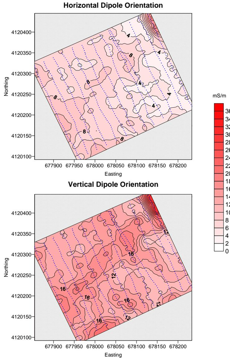
Figure 3 – Spatial pattern of apparent conductivity in an area of Mack fine sandy loam, 1 to 3 percent slopes, measured with the EM38DD meter.
