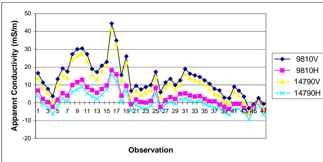
Figure 4 – Spatial pattern of apparent conductivity in an area of Gypsey loam, 3 to 6 percent slopes, measured with the GEM300 sensor operating at a frequency of 9810 and 14790 Hz in the horizontal and vertical dipole orientations.
