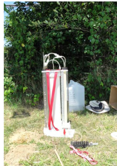
An amoozometer is utilized to measure saturated hydraulic conductivity in soils.
