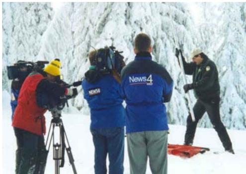
involve taking many core samples to determine the average water content in that area. They measure the snow depth by pushing a metal tube down through the snow pack to the ground and extracting the core. The core sample is weighed to calculate the water content.
