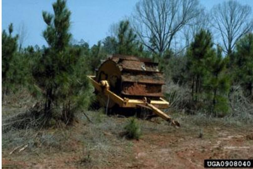
Figure 4. A small rolling drum chopper used to conduct a pre-commercial thinning. Source: David J. Moorhead, University of Georgia, Bugwood.org
